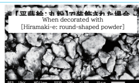
When the fine powder makes it difficult to discern with the naked eye, SEM can be used to clearly identify the metal shapes used.
