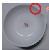
Analysis is possible with as less as one grain of vermillion collected with the adhesive tape
